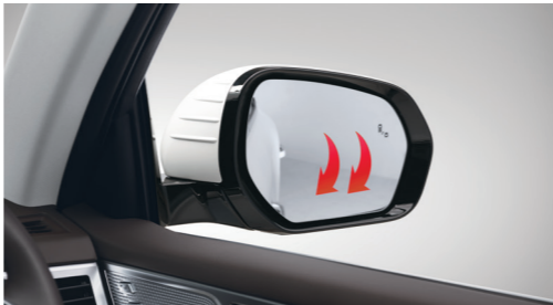
Automatic tilt-down external mirrors when reversing
