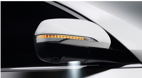
Exterior rear view mirrors with side repeater and puddle lamp
