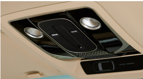
Overhead console with red seatbelt reminder light
