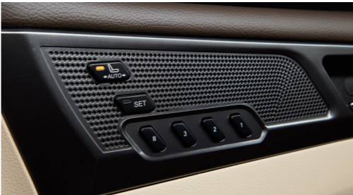
Position memory control system for driver's seating
