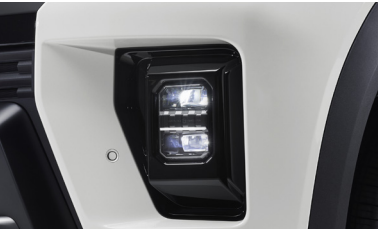
Manual Leveling LED Head Lamps
