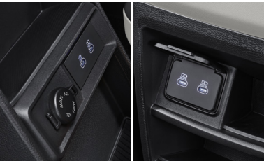
USB Type-C Ports (Front: 1 Charging, 1 Data & Charging / Rear: 2 Charging)
